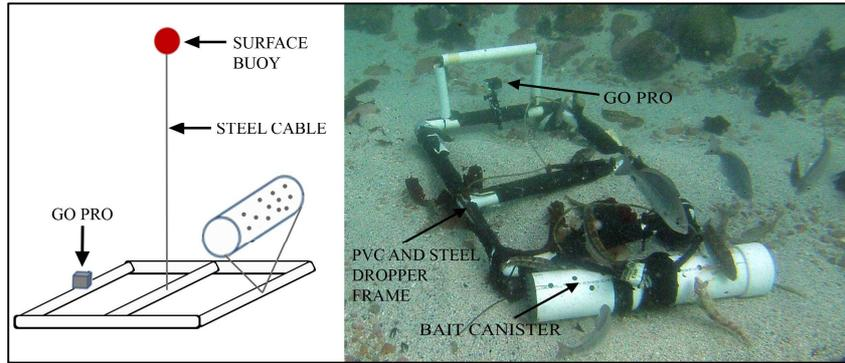
**Figure 2.** Diagram of the baited remote underwater video systems (BRUVS) deployed for the kelp-correlation experiment.
